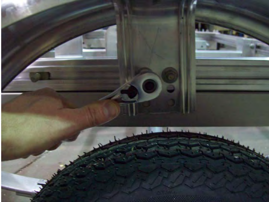
Tighten the nuts on the fender brace.
