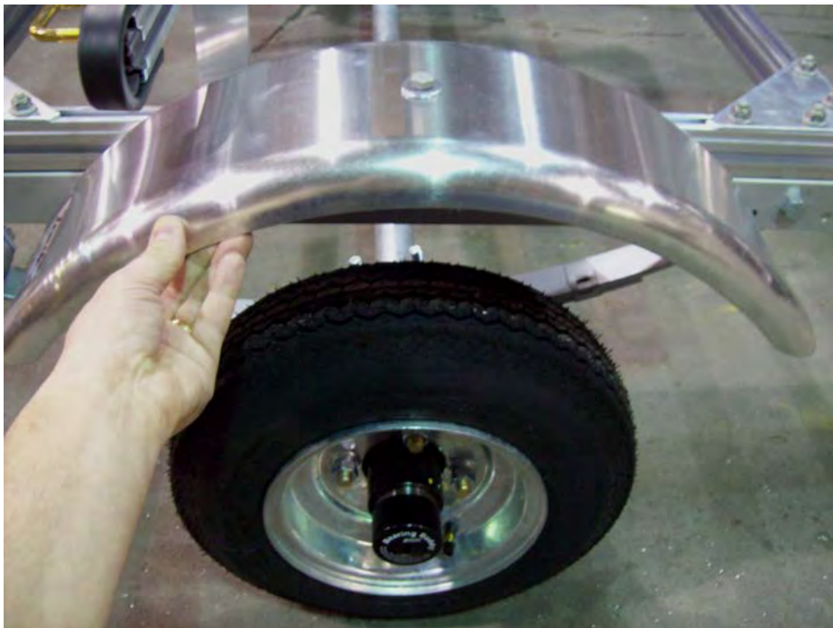
Once fender has been tightened up, center it over top of the wheel.
