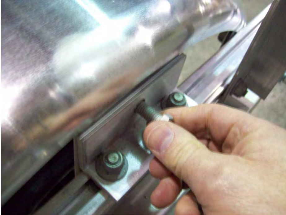
Insert bolt through the back side of the angle bracket.
