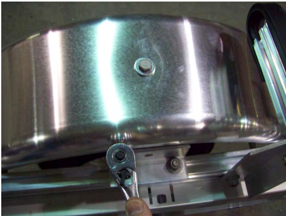
Align the fender bracket with the outside edges of the fender brace. Tighten nuts.
