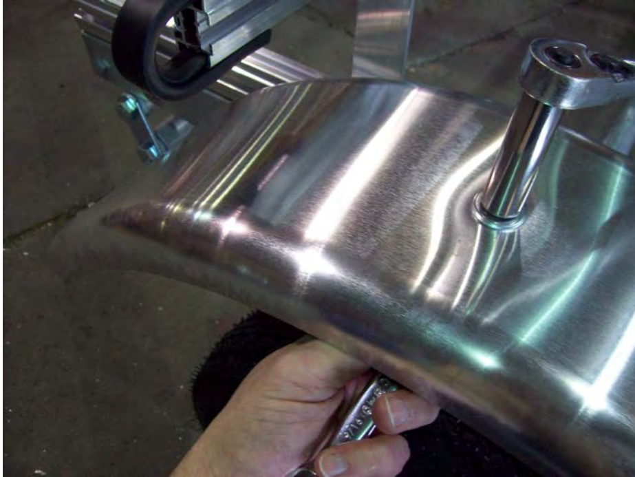
Align fender with side rail and tighten nut.
